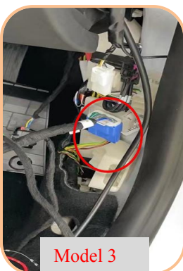
8. Remove the upper cover of the passenger side's footwell
