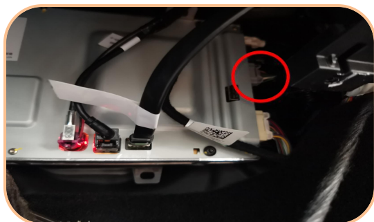
9. Then remove the side cover plate of the passenger side's footwell
