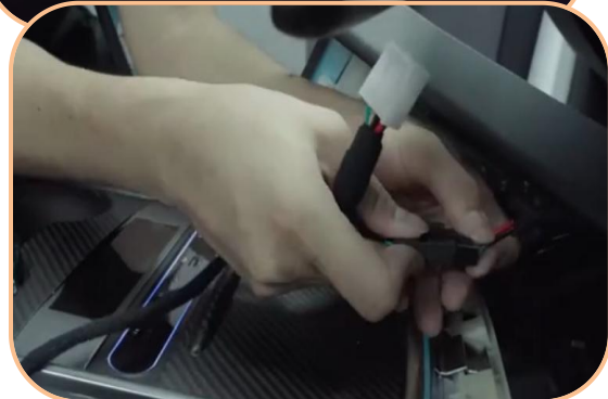
7. Connect harness plug ② to this position (Please skip this step for Intel versions)
