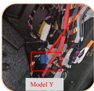
8. Remove the upper cover of the passenger side's footwell
